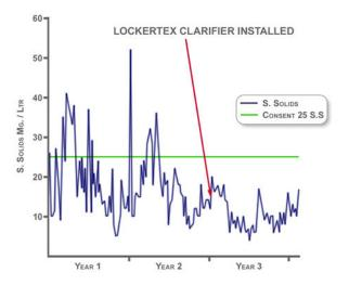
The graph demonstrates the value of Lockertex Clarifiers in reducing peak levels of S.S.
